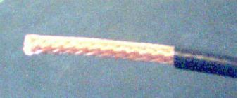
Step 2: Flip the exposed braid back over the insulated part of the coax. Be careful doing this as the braid has to lay smoothly over the coax or the next step will be impossible.
