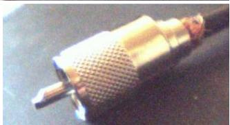
Step 6: Clip away the excess center wire and spin the outer ring forward over the connector housing and the connector is now ready to use.
