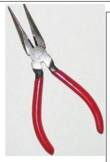
**EVER WISH YOU HAD A THIRD** HAND TO HOLD A PART, OR **HEAT SINK A PART WHILE** YOU WERE **SOLDERING IT. WELL THIS IS ONE EASY WAY** TO DO JUST THAT, JUST STRETCH A **RUBBER BAND ACROSS THE HANDLES OF A**
